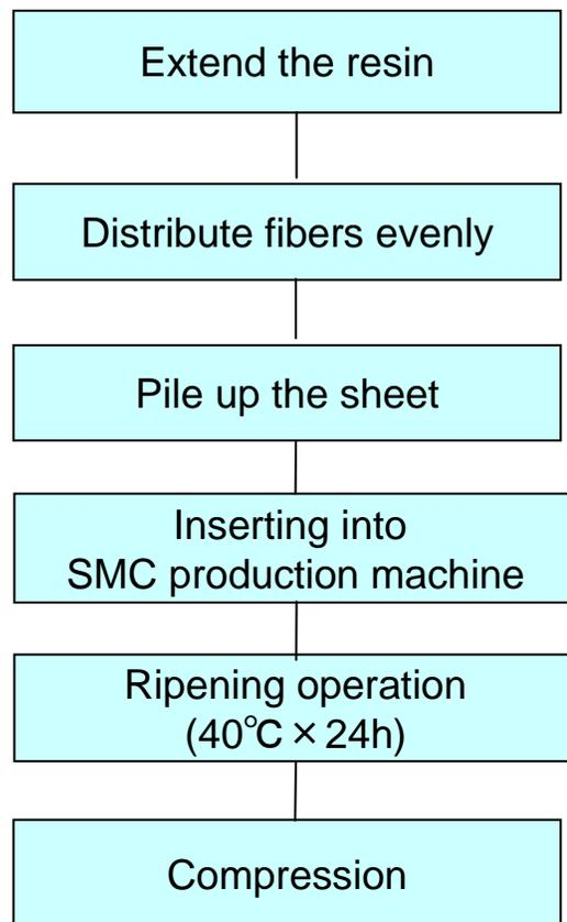
Fig.2 Flow Chart of SMC production
