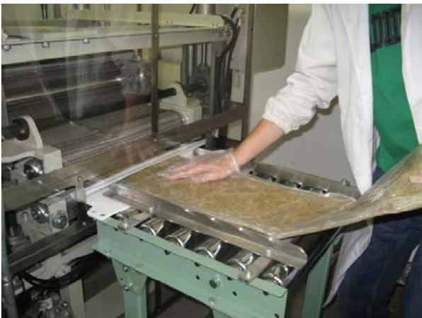
Fig.1 New small SMC production machine
